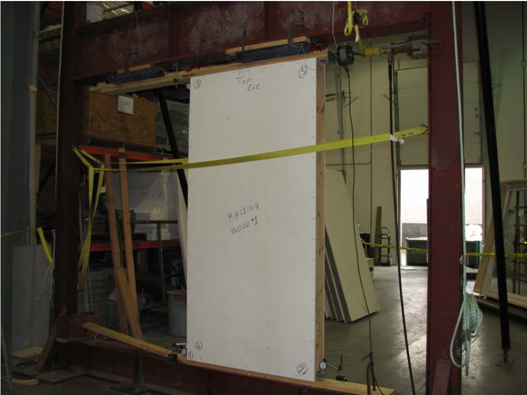
Racking load test setup
