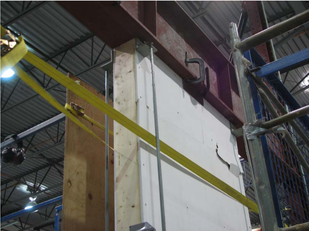
Axial load test setup showing position of compression measurement equipment
